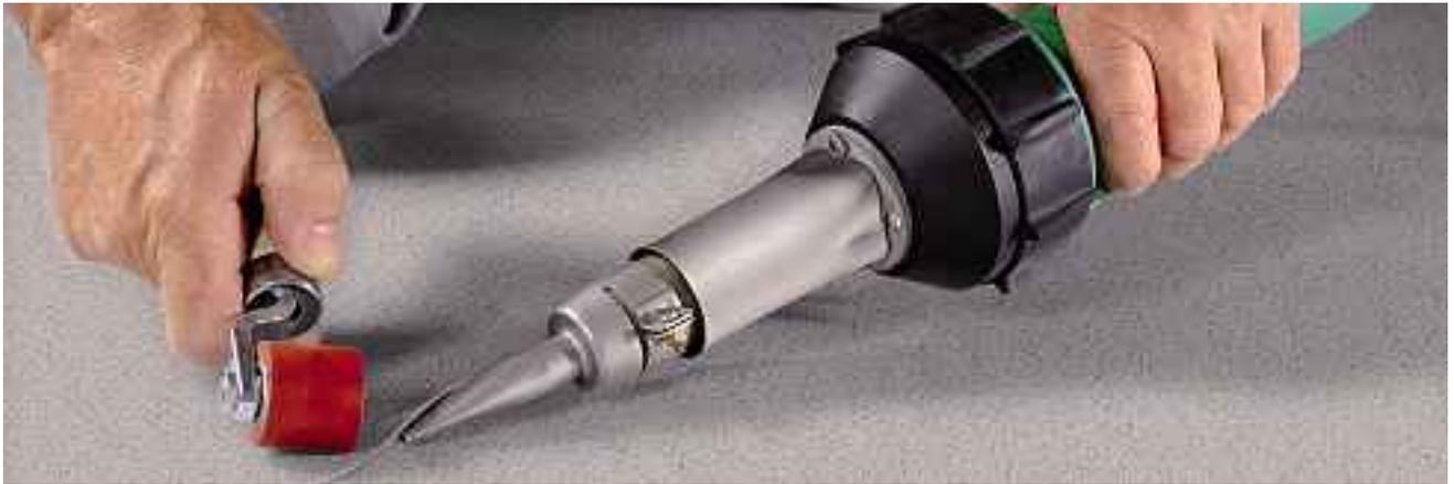
In every roofing system being installed, the Sika PVC and FPO single ply membranes must always be securely welded together with special welding equipment using hot air. The following methods are used for welding – hand welding and automatic welding.
