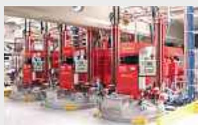
Sika's polyurethane coatings are produced using automated plants with electronically measured and dosed raw materials in stainless steel dissolving mixers. Each production unit has a powerful motor, its own heating and cooling system and an automatic discharging and cleaning system. Products are then packaged in steel drums.
